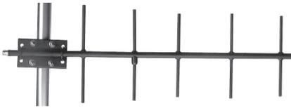
The BMOY UHF models are available in 3 element and 5 element versions. Each version includes models covering 406-440 MHz, 430-460 MHz, and 440-480 MHz. The line also includes a 5 element model covering 470-512 MHz.
